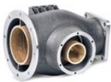
Multi-Material Heat Exchanger | Engineering Material: Stainless + Bronze Dimensions: ø 200 × 400 mm Building time: 22 h Machining time: 55 mins.
