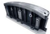
Forming Die (repair) | Die & Mold Material: Hardened Steel Dimensions: ø 1,100 × 425 × 218 mm Building time: 50 mins. Machining time: 10 mins.
